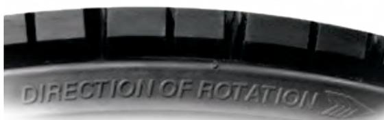
Directional treads should be mounted facing opposite directions to ensure their "direction of rotation" arrows are each pointed to the front of the vehicle. This arrow can be found on the sidewall.
