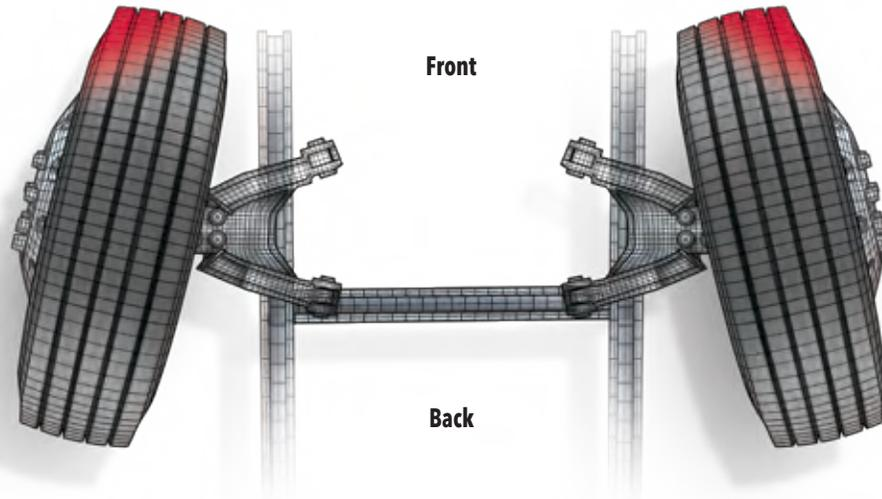
**TOE-IN** The distance between the front of the tires is less than the distance between the rear of the tires.
