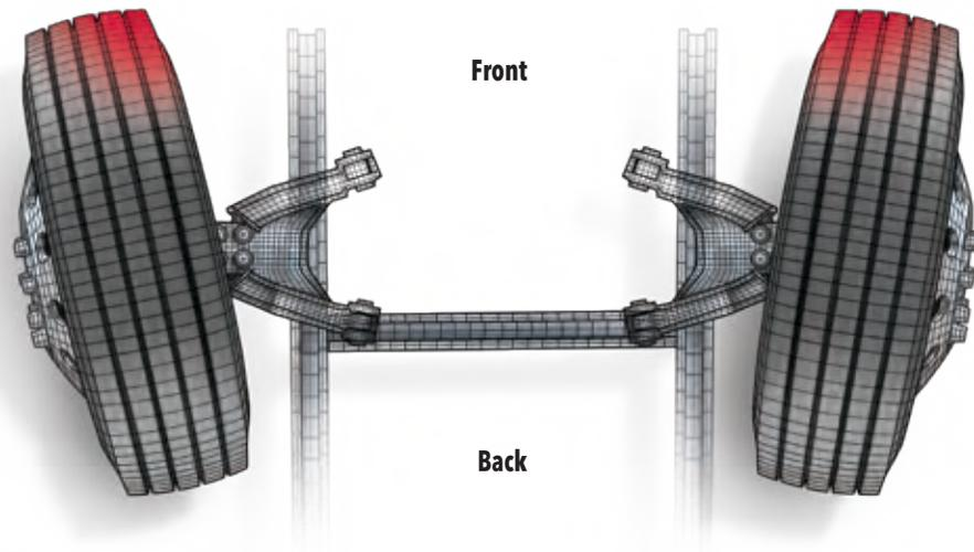
**TOE-OUT** The distance between the front of the tires is greater than the distance between the rear of the tires.
