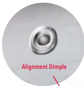
Note: Not all wheel assemblies indicate the point of minimum radial run-out.
