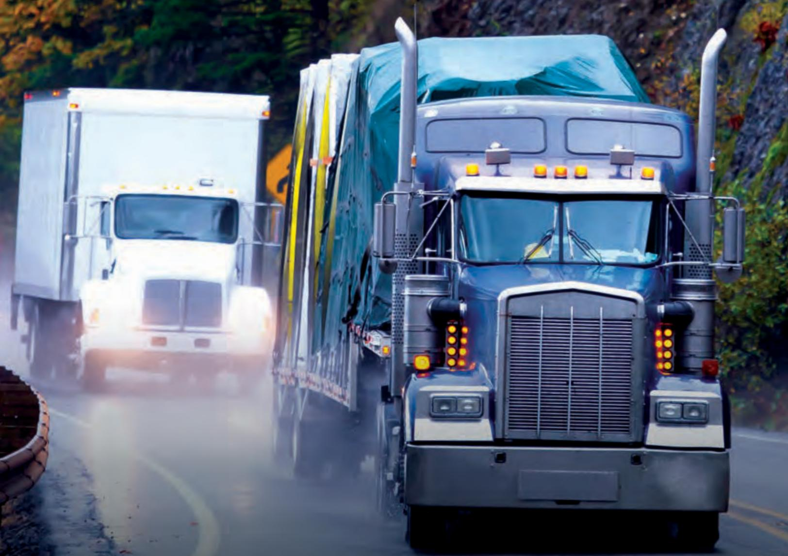
Proper alignment is an important factor in lowering operational costs. Ideally, when a truck is traveling in a straight line, all of the axles are parallel—and perpendicular to the vehicle centerline—and all the tires are rolling in a straight line, too. Not only will tires on a properly aligned vehicle last longer, but some manufacturers suggest that there are significant improvements in fuel economy, component wear, and even driver fatigue.
