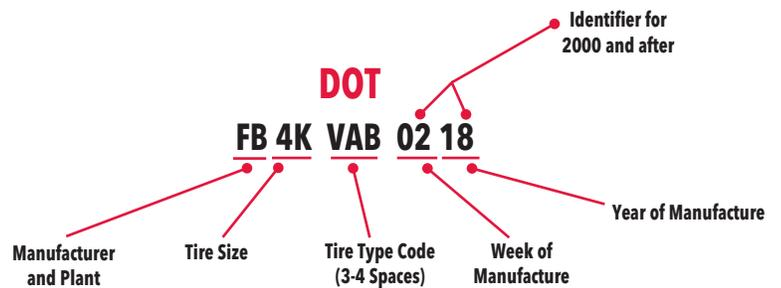
Some manufacturers place an additional code with a specific serial which identifies the specific tire model (a tire type code). This optional number is located on the sidewall opposite the DOT number.
