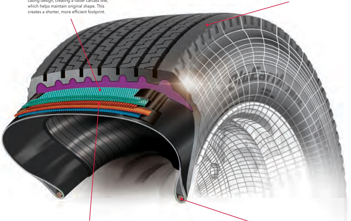
**Zero degree belt**, engineered specifically to provide even pressure across the contact patch, allows for even weight distribution and vastly increased treadlife.
