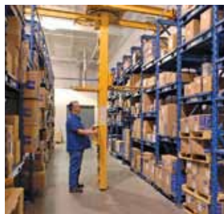
Aisle space requirements are narrower than those required when using a conventional forklift.
