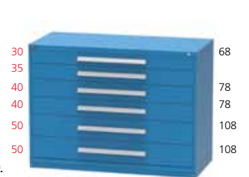
RP2148AL 44 in. (1118 mm) High 6 Drawers 224 Compartments Usable Drawer Heights 3-7/8 in. (98 mm) 4-5/8 in. (117 mm) 5-3/8 in. (137 mm) 7 in. (178 mm) 747 lbs. (339 kg.) Shipping Weight
