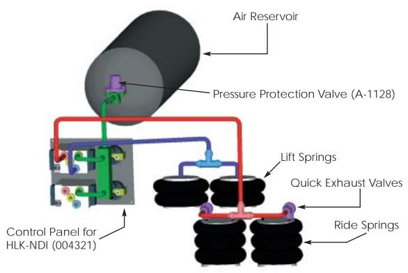
\*Note: Schematic only shows connections for one suspension.
