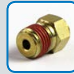
HP1099 MALE PIPE CONNECTOR Material: Brass Fitting End A: 1/4" OD Tube Fitting End B: 1/4" (-4) NPT Male (Pre-Applied Sealant) NON-DOT
