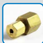
HP1120 FEMALE PIPE CONNECTOR Material: Brass Fitting End A: 1/8" OD Tube Nylon Fitting End B: 1/8" (-2) NPT Female NON-DOT
