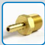
C10568 MALE PIPE CONNECTOR Material: Brass Fitting End A: 1/8" ID Tube Fitting End B: 1/8" (-2) NPT Male
