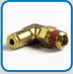
HP1122 MALE PIPE 90° SWIVEL ELBOW Material: Brass Fitting End A: 1/8" OD Tube Fitting End B: 1/8" (-2) NPT Male (Pre-Applied Sealant) NON-DOT
