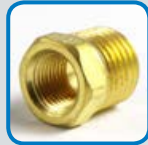
HP1096 BUSHING Material: Brass Fitting End A: 1/4" (-4) NPT Male Fitting End B: 1/8" (-2) NPT Female
