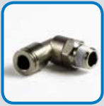
HP1019 MALE PIPE 90° SWIVEL ELBOW Material: Nickel Plated Brass Fitting End A: 1/4" OD Tube Fitting End B: 1/8" (-2) NPT Male (Pre-Applied Sealant) NON-DOT
