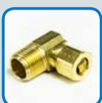
HP1236 MALE PIPE 90° ELBOW Material: Brass Fitting End A: 3/8" OD Tube Brass/Copper/Aluminum Fitting End B: 3/8" (-6) NPT Male NON-DOT
