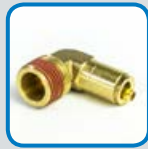
HP1245 MALE PIPE 90° ELBOW Material: Brass Fitting End A: 1/4" OD Tube Fitting End B: 3/8" (-6) NPT Male (Pre-Applied Sealant) NON-DOT
