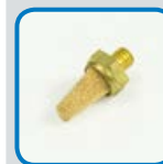
C10833 POROUS BRONZE AIR SILENCER Material: Bronze Fitting End A: 10-32 UNF Male Filtration: 40 µm Max Rated: 2 CFM @ 90 psi
