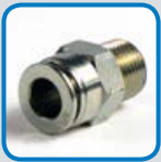
HP1098 MALE PIPE CONNECTOR Material: Nickel Plated Brass Fitting End A: 1/4" OD Tube Fitting End B: 1/8" (-2) NPT Male NON-DOT
