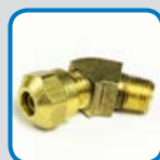
C10591 MALE PIPE 45° ELBOW Material: Brass Fitting End A: ¼" OD Tube Nylon Fitting End B: 1/8" (-2) NPT Male DOT
