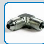
C3468 90° ELBOW Material: Steel Fitting End A: ¼" (-4) JIC Male Fitting End B: 1/8" (-2) NPTF Male
